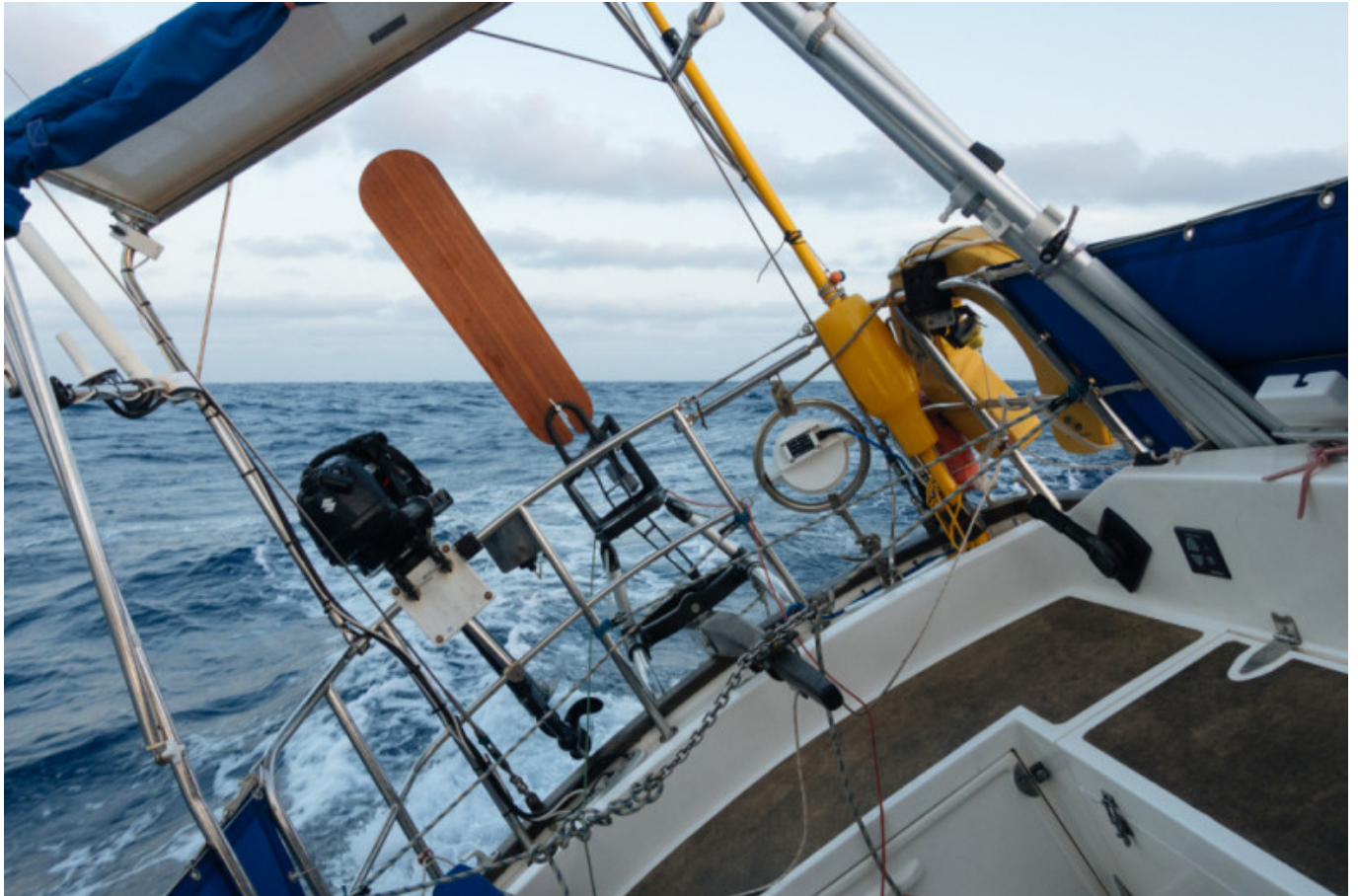
self steering & towed generator doing their jobs
